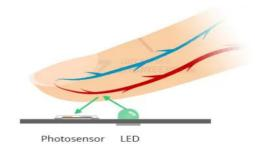
The oxygenated hemoglobin in arterial blood has the property of absorbing green light. The redder the blood (the higher the hemoglobin), the greater the absorption of green light. With each heartbeat, blood is pumped through the finger, causing a change in the amount of reflected light, which in turn produces a waveform at the photosensor's output.
